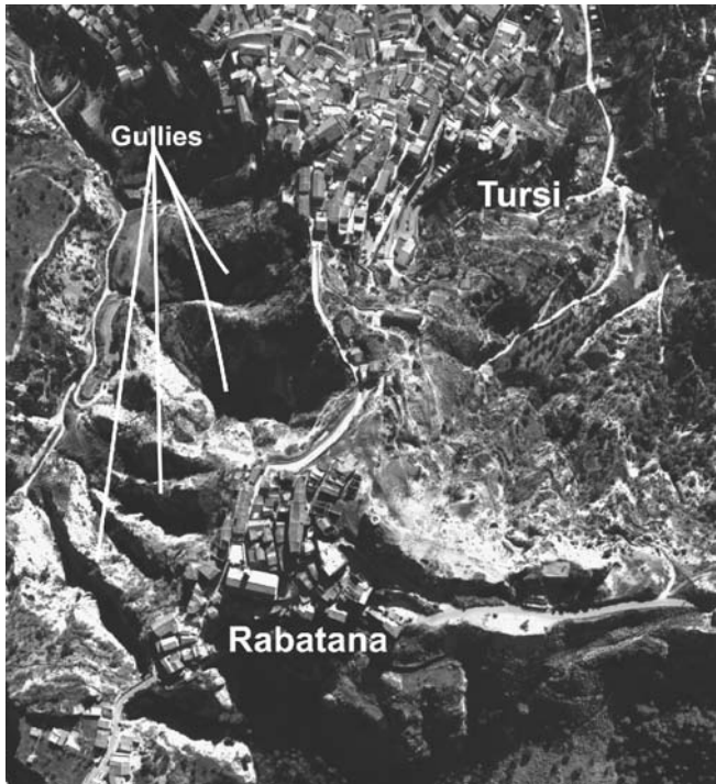
Fig. 4 Aerial view (scale 1:2,000) of the study area with evidence of deep gullies and steep slopes that surround the urban areas of Tursi town and its oldest nucleus, called “Rabatana”
